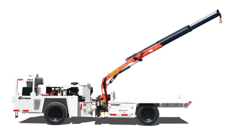
Getman materials transport vehicles are versatile underground carriers designed to move materials throughout a mining operation reliably and efficiently, ensuring loads are delivered where they are needed when they are needed. Available crane packages maximize the opportunity for utilization throughout underground operations while increasing efficiency and productivity during loading and unloading scenarios.
