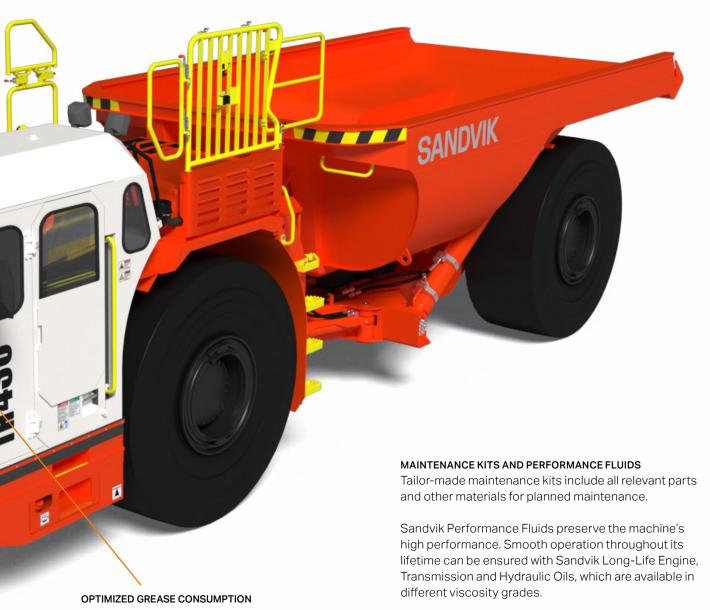
The standard Automatic Central Lubrication System optimizes grease consumption and extends the life of the bushes and bearings. Activated by Sandvik Intelligent Control System when park brake is released, hard to reach areas are well lubricated and service time is reduced.
