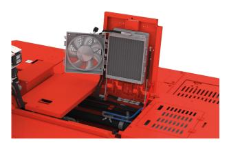
The air conditioning system is directly driven off the engine for increased reliability and it is independent of other hydraulics for easy troubleshooting.
