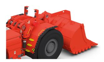
Improved boom locking mechanism enables one-handed operation and maintaining 3-point contact. The boom uses robust solid floating pins with a M30 pull out thread for easier pin removal, along with new bush lip sealings to prevent the ingress of dirt, reducing wear. The loader is equipped with more greasing points in the boom geometry, well protected grease lines and automatic central lubrication system with increased capacity for longer time between refilling.
