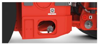
The cold side includes a filter station for engine and brake filters with ground level access. An efficient Power Core engine filter is housed well within the frame, and it utilizes an ejector valve system for increased filter lifetime.
