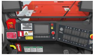
To minimize the need to move around the machine or use special tools, the 7" color display in the operator's compartment provides service information, easy system diagnostics and alarm log files.
