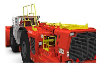
Engine coolers, side coolers for transmission, brakes and hydraulics, each have a swing out fan for easy cleaning.
