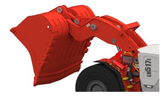
The boom lock is integrated into the front frame and allows one-handed operation maintaining 3-point contact. The boom uses robust solid floating pins with a M30 pull out thread for easier pin removal, along with bush lip sealings to prevent the ingress of dirt, reducing wear. The loader is equipped with more greasing points in the boom geometry, well protected grease lines and automatic central lubrication system with increased capacity for longer time between refilling.
