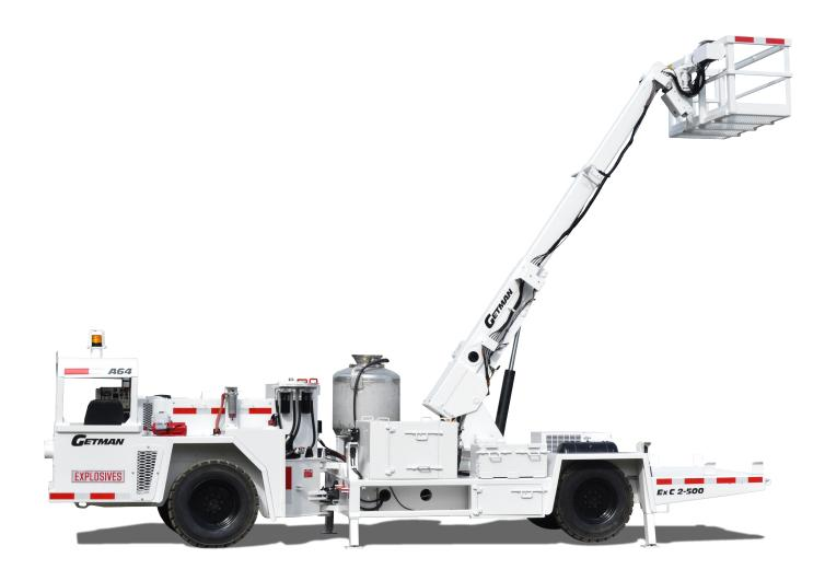
Getman explosives chargers are versatile explosives charging vehicles designed to work in development drifting, production charging, up-hole charging applications and more. They can be configured for ANFO charging, emulsion charging, or both.
