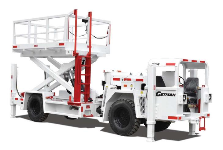
Getman scissor lifts are a key component of underground mining operations, supporting electrical installations, ventilation fan and ducting installations, pipe installations, ground support operations and explosives charging.
