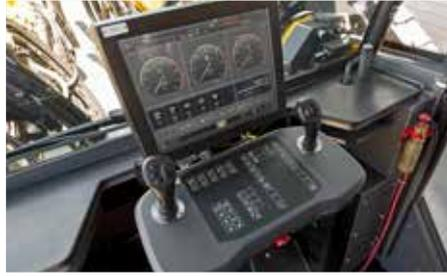
The control system is easy to learn and maximizes the performance with faster boom positioning and optional fully automated drilling.
