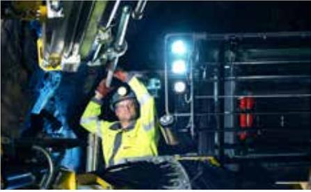
With the unique safe bolting boom function there is no need to step in front of the rig under unsupported rock during bolt installation. All service points are accessible from ground level.
