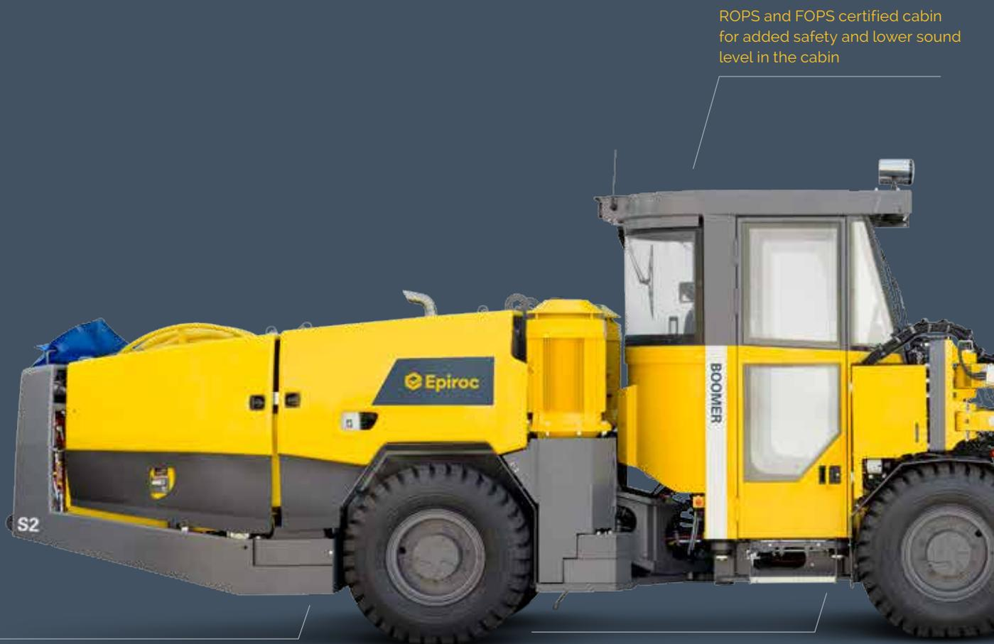
ROPS and FOPS certified cabin for added safety and lower sound level in the cabin
