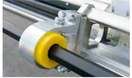
The new feeds feature interchangeable drill steel bushings which means that you can use either rubber or steel bushings without changing holder.
